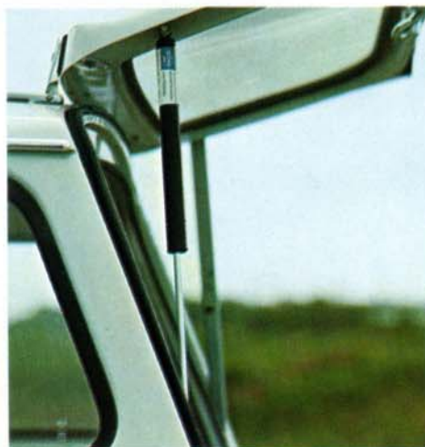
A gas cylinder assist makes lifting the top of the door a snap.
